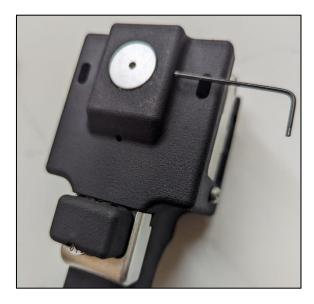
Removal of upper sealing plug and pad assembly.
