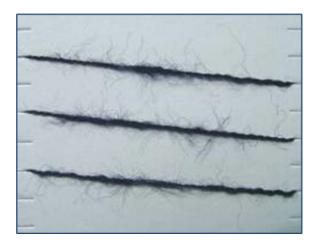
The 111 Series splicers make a joint of the "ends-opposed" form. This type of splice generally has excellent appearance, whether used on "wellbehaved" yarns such as multifilament nylon, or on more difficult yarns such as those made from staple blends.
