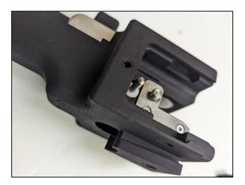
Removal of lower sealing plug and knife drive.
