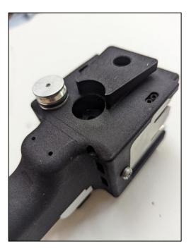
Removal of lower sealing plug and knife drive.
