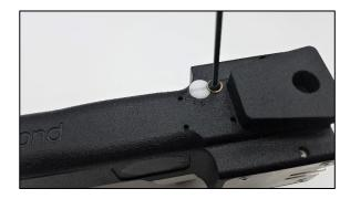
Removing flow control assembly
