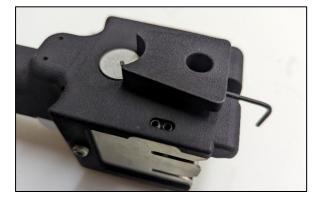
Removal of lower sealing plug and knife drive.
