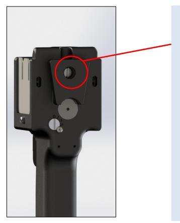
To release the splicing chamber, remove the single fixing screw Item 705 from the rear of the splicer body, when the splicing chamber can be lifted clear of the splicer.
