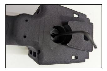
Removal of lower sealing plug and knife drive.
