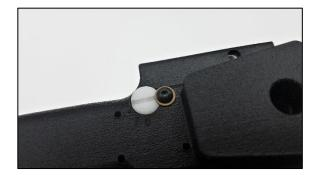
See the flow adjustment screw on the back of the splicer – the white circle.
