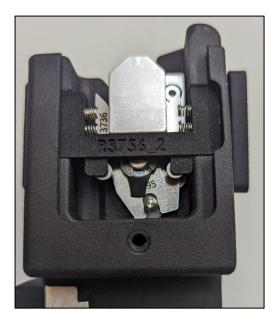
All splicers of the 182 range are capable of dealing with a wide range of yarn counts. Yarn clamp pressure is a contributor to splicing efficiency.
