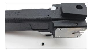
Removing flow control assembly
