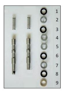
Removing valves, spacers, and O-rings
