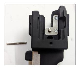
Removal of lower sealing plug and knife drive.
