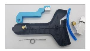
Here is the splicer with its principal components disassembled: Body shell (with lower compression fitting still attached) Trigger (with closure pad still attached) Trigger return spring. Blue air supply tube. Complete splicing unit (at extreme right)
