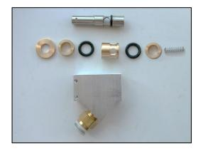
This photograph shows the splicer unit completely dismantled. Top: valve, Item 1606 with oring, Item 1651 From left: Retaining disc, Item 1601. Brass spacer, Item 1602 O-ring, Item 218 Shell, Item 1607, O-ring, Item 218 Brass spacer, Item 1602 Return spring, Item 787 Bottom: valve body, Item 1600 with Connector, Item 1618
