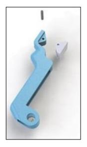
If required, press out the pad retaining pin, Item 1605, and separate the trigger Item 1614 and closure pad Item 1610
