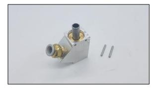
With the two pins removed, removal of the inner components – the final dismantling of the splicer unit - can commence.
