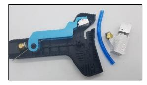
Lift away the trigger assembly, together with the chamber pad. Keep the assembly as one unit, unless you need to remove the chamber for maintenance or replacement.
