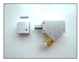
Remove the splicing chamber. With a small tool, press the chamber securing pin, Item 1604, until it slides out. The chamber can then be removed from the Valve, Item 1606.
