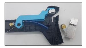
Then release the feed tube from the upper compression fitting. This will permit the removal of the air union and feed tube.
