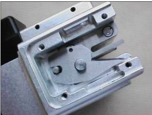
Figure 35. Knife spring removed
