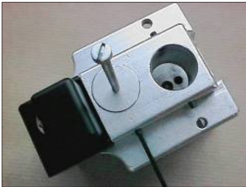
Figure 39. Removal of lower sealing plug
