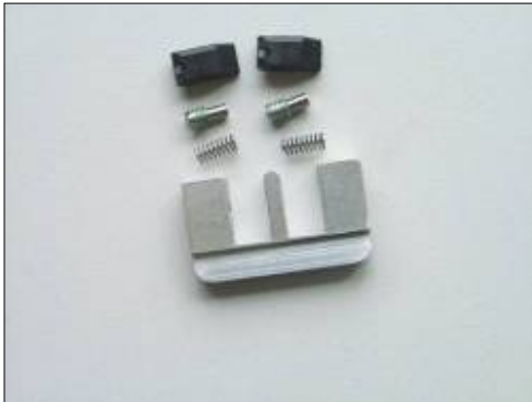
Figure 31. Yarn clamp assembly dismantled
