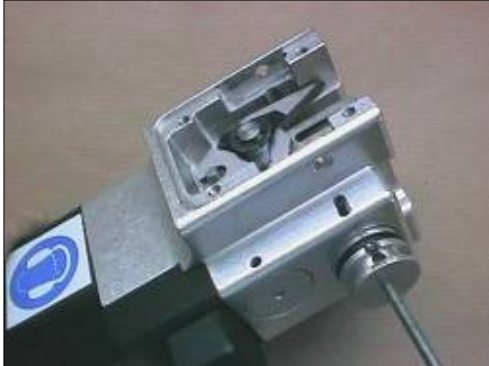
Figure 20. Upper sealing plug removal
