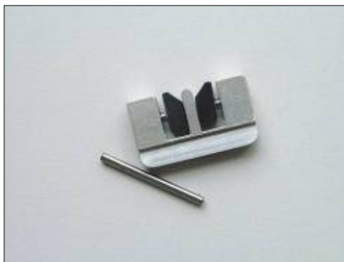
Figure 29. Stabilising pin out
