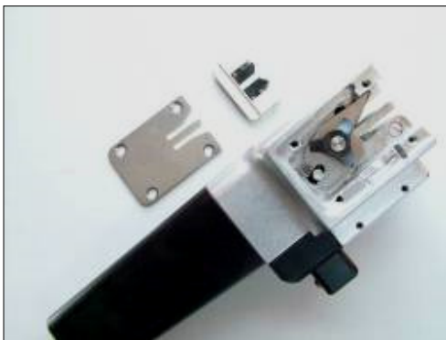
Figure 26. Yarn clamp holder removed
