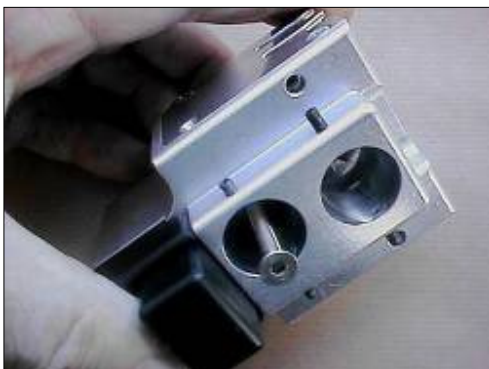
Figure 43. Remove knife drive piston
