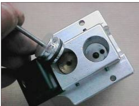
Figure 40. Knife piston plug removal
